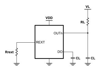
**Switching Characteristics Test Circuit**
