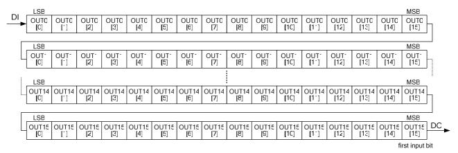
16x16-bits M-PDM data are transmitted into a device for each scan according to the format illustrated above. The first input bit is the most significant bit of OUT15.
